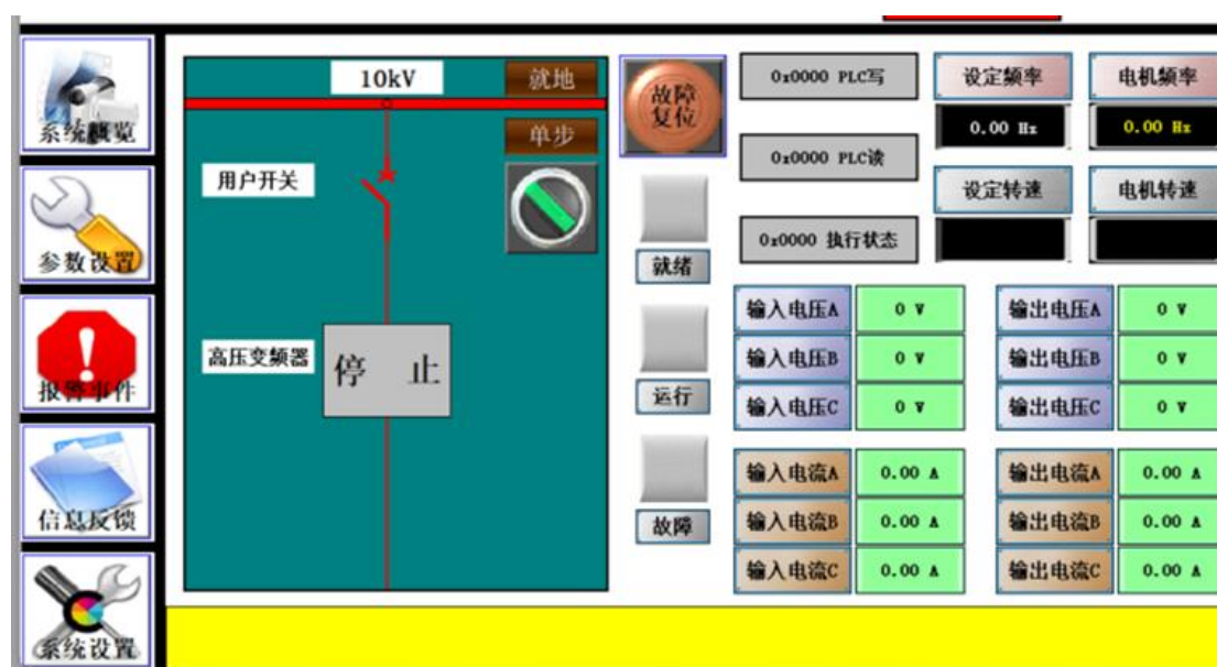
Figure 2-4 Schematic diagram of the control part of the high-voltage inverter
