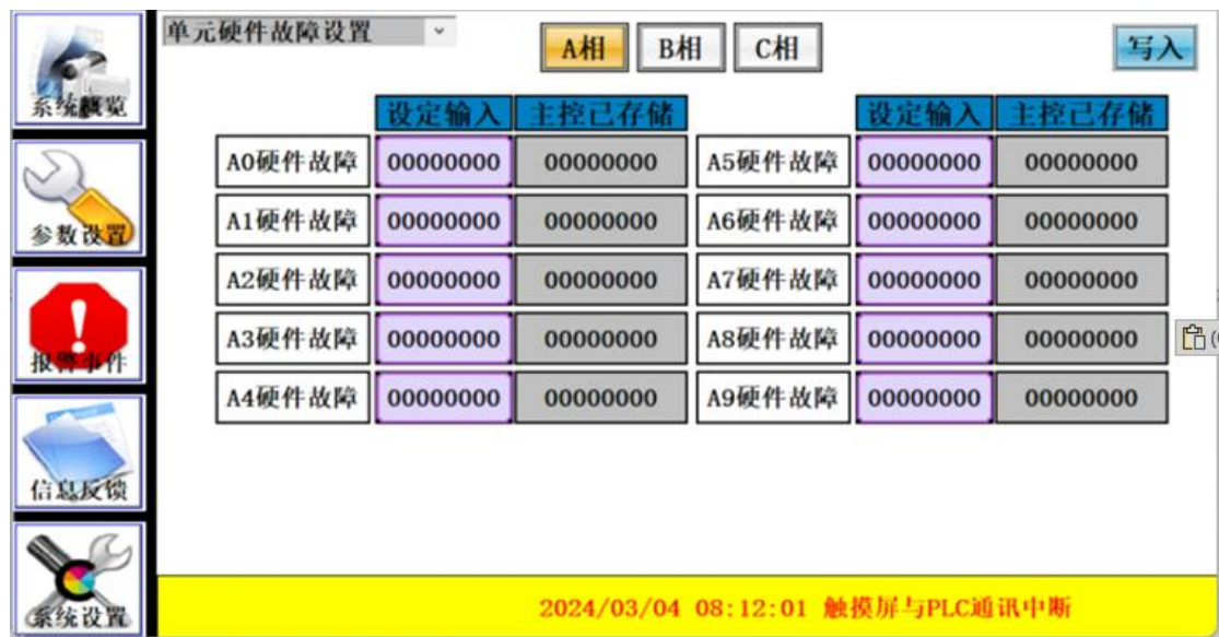
Figure 3-10 Unit Hardware Fault Setting Interface
