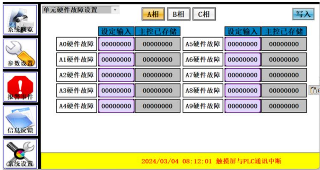
Figure 3-10 Unit Hardware Fault Setting Interface
