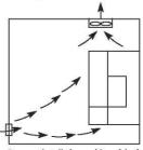
Incorrect installation position of the fan
