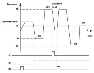
Action instruction: ① Press K1 to startup the inverter and the potentiometer will set output frequency.
