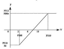
Introduction: P300=2 FIV minimum voltage input: 2V (inverter regards signals below 2V as invalid signals):
