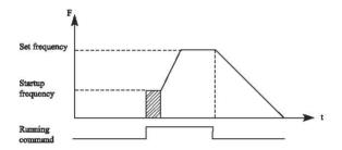
Start frequency is the initial frequency when inverter starts. For device with heavy load or requires large starting torque, increasing start frequency can make start easier. However, if the start frequency is too high, it may cause over current protection.
