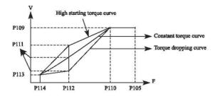
P109: V/F maximum voltage, V/F maximum voltage can be set according to the motor connected. Generally, it will be set at the rated voltage of motor. When motor is very near to inverter, usually within 30m, it should be set at a higher value.
