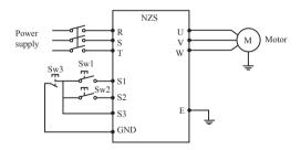
Use S1, S2, or S3 as input terminal for external signal
