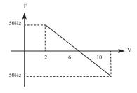
Example 2, upper computer output 4-20mA, and controls running of inverter Output frequency is 100Hz-0Hz
