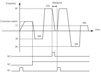
Action instruction: ① Press K1 to startup the inverter and the potentiometer will set output frequency.
