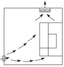
Incorrect installation position of the fan
