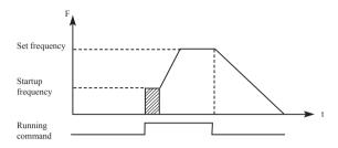
Start frequency is the initial frequency when inverter starts. For device with heavy load or requires large starting torque, increasing start frequency can make start easier. However, if the start frequency is too high, it may cause over current protection.
