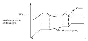
100% current is the rated current of inverter, when P409 is set to be 0, then accelerating torque limit is invalid, and it does not have protecting function.
