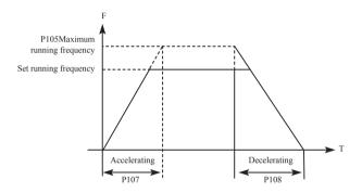
The Default Acc/Dec time is the primary Acc time/ Dec. time. Other Acc time or Dec time can be selected via external terminal.
